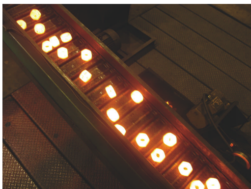
Nuts, still orange-hot, after being formed.
