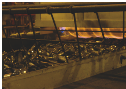
Hardening involves temps of up to 1,570 °F.
