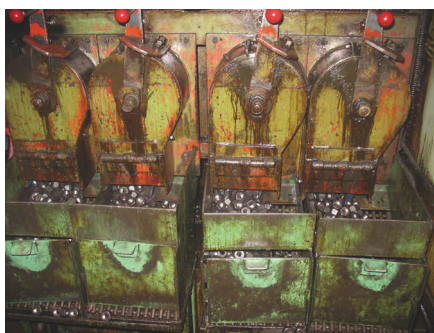
Tapping machinery threads the nuts.
